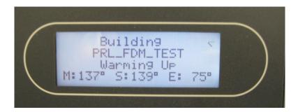
Once the machine is warmed up, your part will immediately begin building. Watch it for a couple of minutes to make sure that the build starts without issues. Post your FDM confirmation card on the front of the machine with the clipboard.
