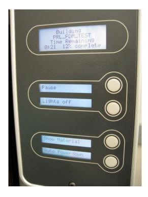
Most parts that will be built on this machine will require many hours of build time. **Auto Powerdown** should be used to prevent overheating and excessive wear on the machine. Once your part has begun building successfully, press the button next to "**Auto Powerdown**", and when prompted, turn **OFF** the machine in the lower right corner. The machine will continue running until it has completed your build and completed its cool down cycle.
