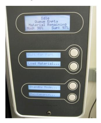
If the machine is at room temperature, it will take about 30 minutes before it has come to temperature and can begin building. There are no adjustments to be made—the required temperatures are hard set into this machine.
