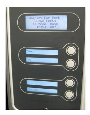
Once you've told the machine that a build base is in place, the machine mode will be "Waiting for Part".
