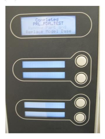
The door will have unlocked itself, and you can open the door and remove the black build base. If the machine is still on, the surfaces inside the machine will be **HOT**! Even if you used Auto Power down and the machine is cold, you should not touch <u>anything</u> inside the machine except for the blue tabs holding the model base in place and the black build base.
